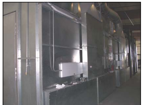
TECON Series 5000 side downdraft, positive pressure, heated paint booth.
