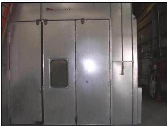
TECON Series 5000 side downdraft, positive pressure, heated paint booth.
